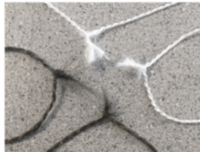
ends together splicing
